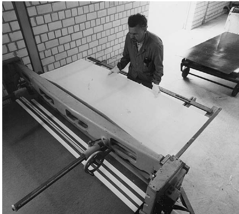
Cutting Palusol Fireboard with guillotine shears.
