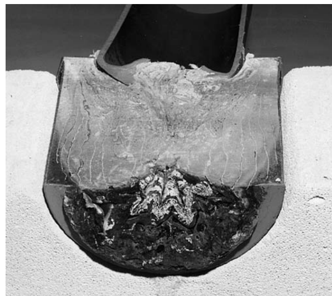
Fire softens the pipe; the expanding sodium silicate closes it and fills the entire space.
